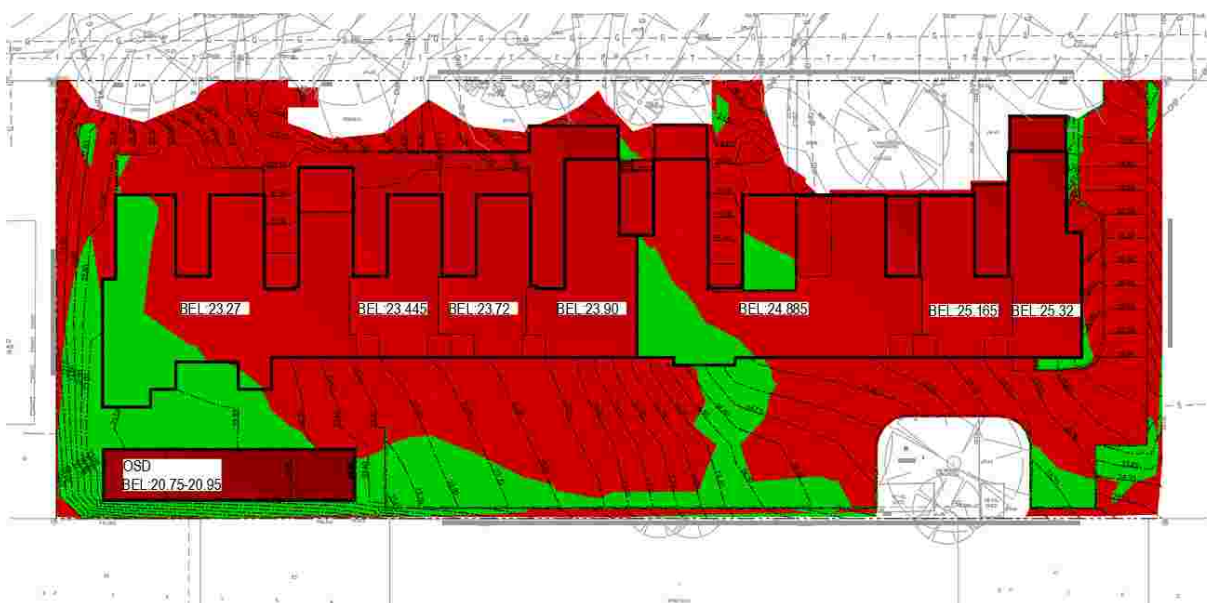
Figure 4: Bulk earthworks cutting and filling Plan. Henry & Hymas 2024
